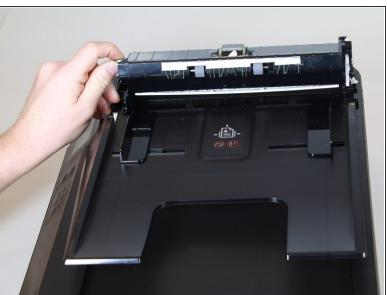
Lift the green tab to remove the fax feeder from the printer.
