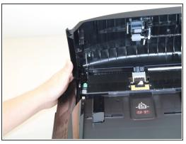
• Use the plastic opening tool to unclasp the hinge that holds the feeder cover.
