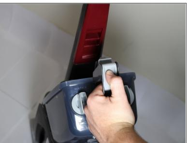
Push the button on the top of the clean water/solutions tank and pull on the handle below the button simultaneously. The tank should easily swing out.
