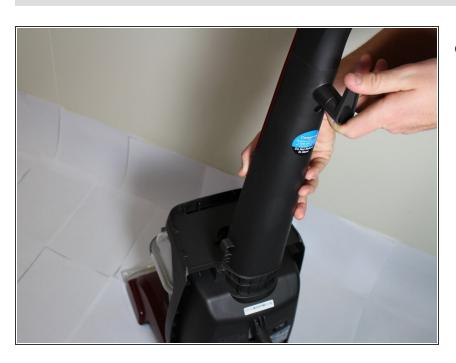
Pull the handle upwards. It should freely slide away from the base of the machine.
