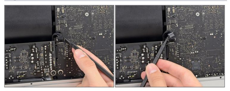
• Use the tip of a spudger to push each side of the power supply control cable connector and gently *walk* it out of its socket.
