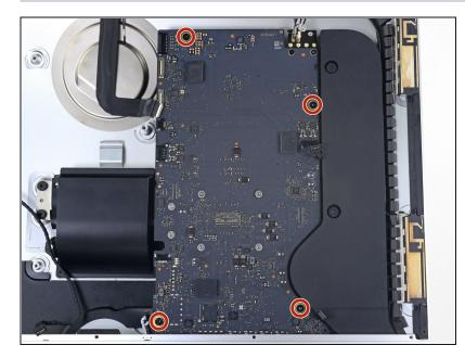
• Remove the four 7.3 mm T8 Torx screws securing the logic board to the rear enclosure.
