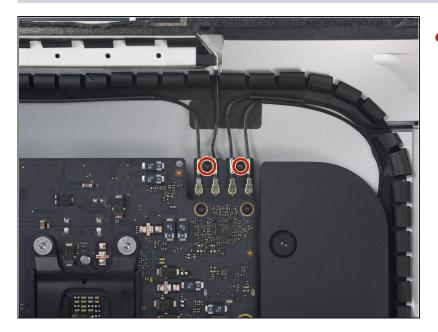
• Remove the two 4.0 mm T5 Torx screws securing the four antenna connectors to the AirPort/Bluetooth card.
