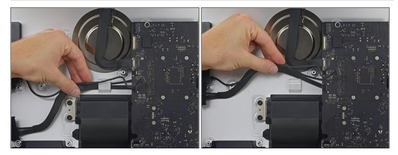
• Similarly to the previous step, de-route the SATA and power cables by pulling the braid straight up out of the retaining clip.
