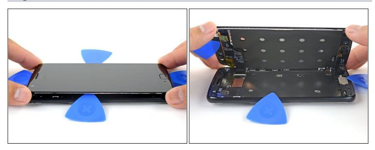
⚠ Do not try to remove the screen yet—it is still attached to the phone by delicate flex cables.
