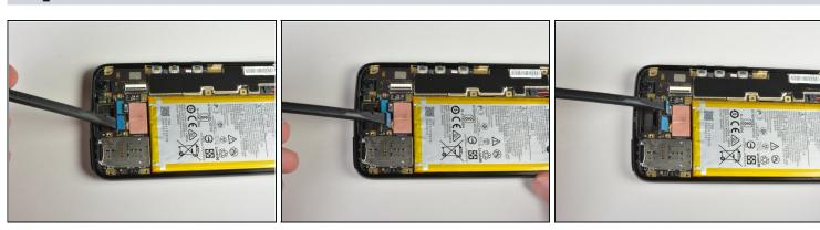
• Use flat edge of the spudger to pry up the two blue connectors near the top of the device.
