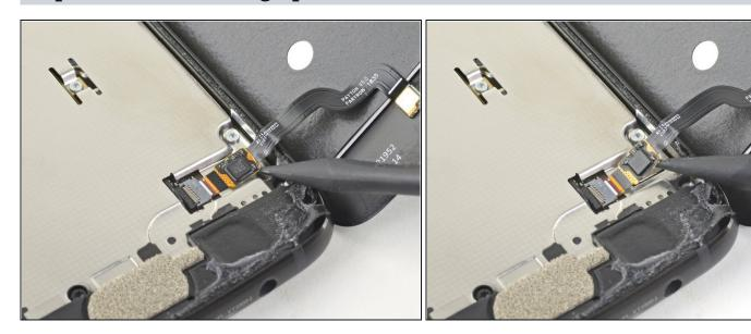
• Slide the point of a spudger underneath the fingerprint sensor cable and gently pry up to loosen the cable from the phone.
