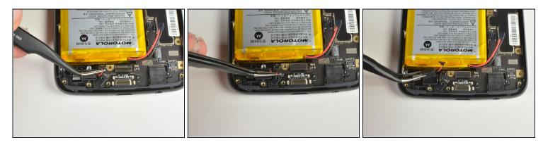
• Using a pair of <u>tweezers</u> disconnect the vibrating motors connector near the bottom of the device.
