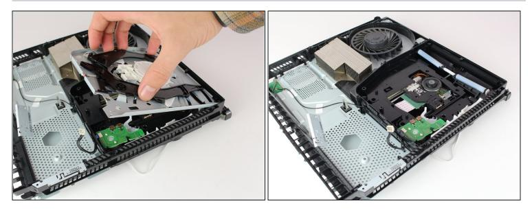
• Remove the disk drive out by pinching on either side of the two black plastic "claws" and lifting up with your hand.
