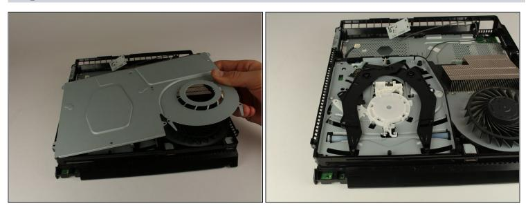
• Remove the metal plate by grabbing the edges and lifting up with your hands.
