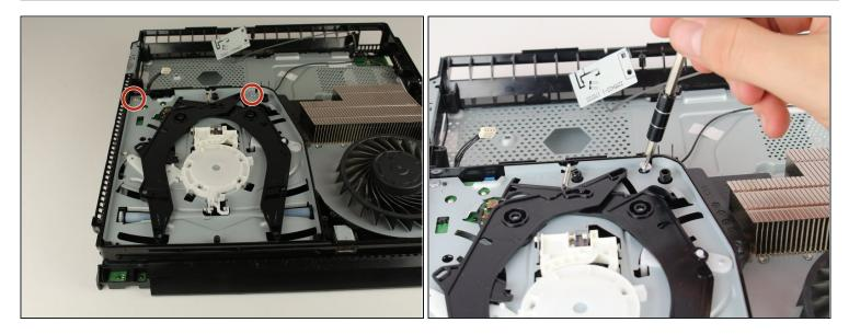
Unscrew and remove the two 3.0mm screws using a PH000 screwdriver with a counterclockwise motion.
