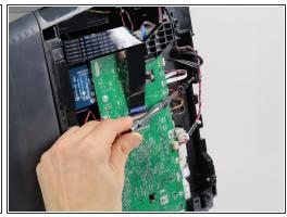
Remove two screws 13mm screws with a T9-Torx screwdriver by rotating them counterclockwise.
