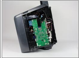
Gently remove the left side panel by placing your palm flat against the surface and pulling down.
