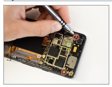
• Remove the two 2.5 mm PH00 screws.
