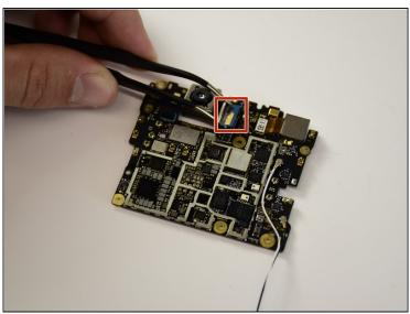
• Remove the ribbon connector that connects the camera lens to the motherboard by grabbing it with tweezers and lifting up.
