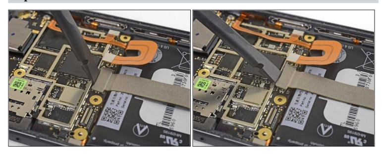
• use the flat end of a spudger to disconnect the charging assembly connector from the motherboard.
