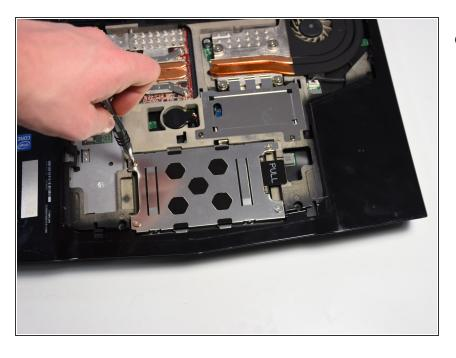
Use Phillips #1 screwdriver to loosen the four screws on the hard drive enclosure.
