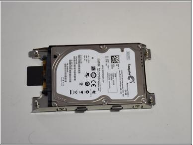
Once the screws are loosened use the "PULL" tab to remove the current hard drive from the computer.
