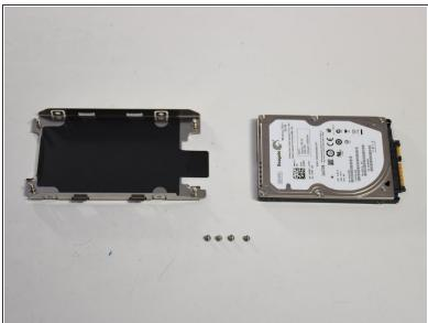
Remove the four small screws indicated to remove the casing to the hard drive.
