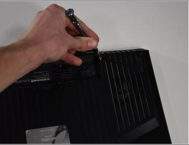
Remove the two 4-mm screws that hold the compartment door to the rest of the computer using a PH#0 screwdriver tip.
