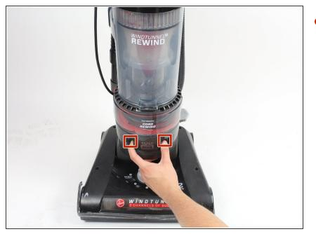
Locate the filter housing which is placed near the bottom of the vacuum
