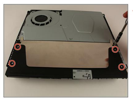
Remove the four 16mm Philips screws holding the power supply in place.
