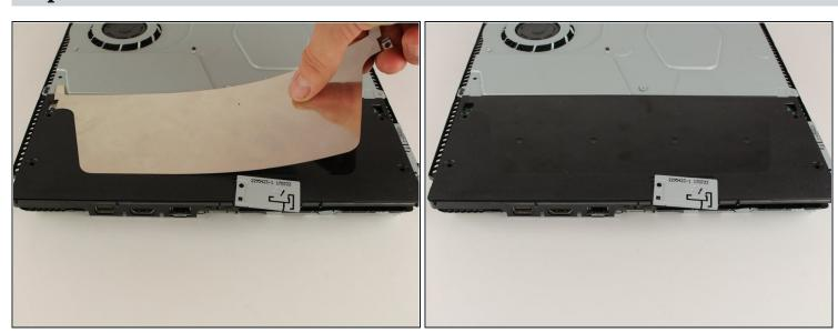
Remove the metal sheet from the top of the power supply by grabbing and lifting up with your hands.
