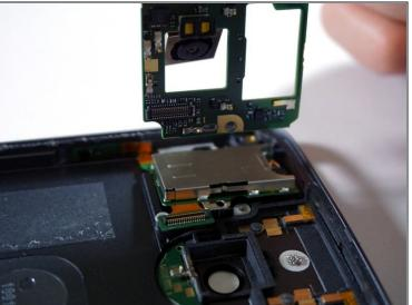
• Detach the connection on the bottom of the motherboard.
