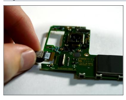
Remove the front facing camera by pulling it out of the locking port.
