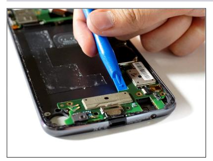
Place a plastic opening tool under the edge of the motherboard.
