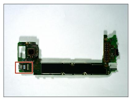
• Identify the ribbon connector that is associated with the front facing camera.
