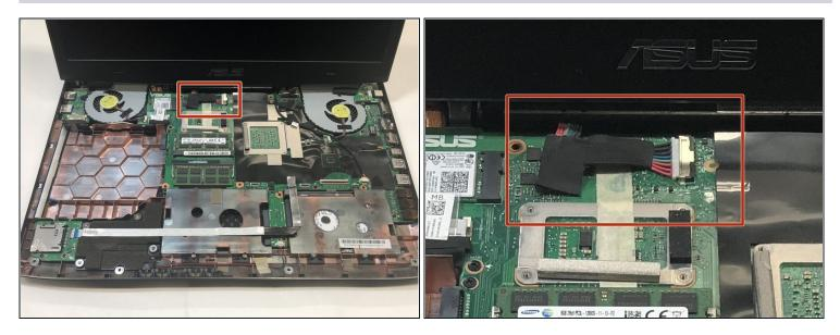
• Use a pair of <u>tweezers</u> to carefully disconnect the pin connector.
