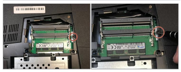
• Use a Phillips 1 Screwdriver to remove the 5 mm screw that is located underneath the back panel.
