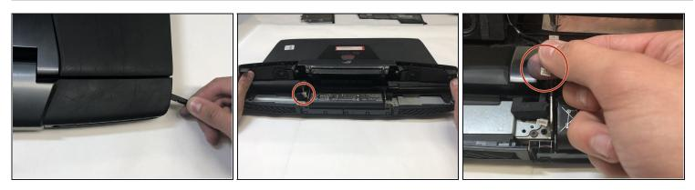
• Use a nylon spudger to carefully pry the top back panel off.
