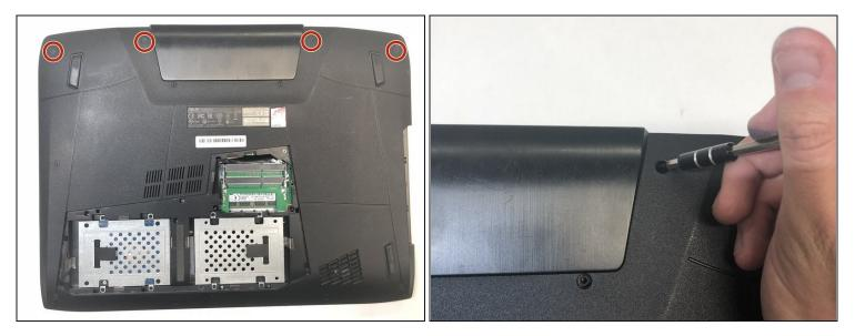
• Use a Phillips 1 Screwdriver to remove the top four 8.5 mm screws.
