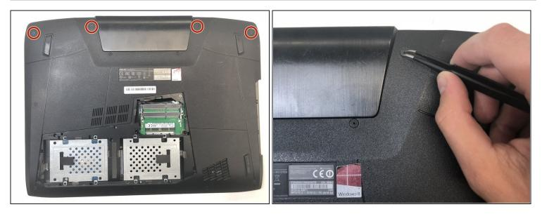
• Use a pair of <u>tweezers</u> to remove the top four rubber stoppers found on the bottom of the laptop.
