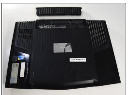
Remove the battery by sliding the latch to the left and pulling the battery up.
