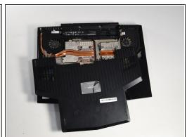
• Slide the compartment door towards the front of the computer and lift.
