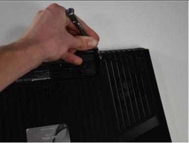
Remove the two 4-mm screws that hold the compartment door to the rest of the computer using a PH#0 screwdriver tip.
