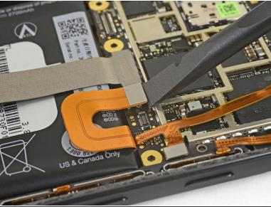
Use the flat end of a spudger to disconnect the battery connector.
