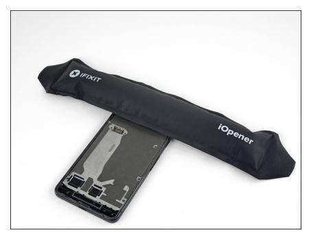
Apply a <u>heated iOpener</u> to the proximity sensor on the top edge of the midframe for two minutes to soften its adhesive.
