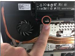
• Use a Phillips #0 screwdriver to remove the two 3mm screws holding the fan in place, then unclip the electrical connection using tweezers.
