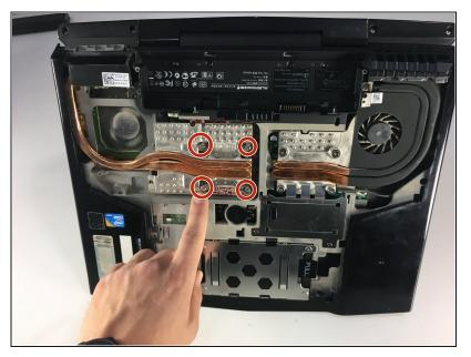
Remove the heat sink by loosening the 4 screws with a Phillips #0 screwdriver.
