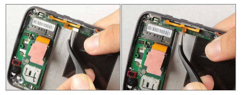
• Remove the golden connector attached to the volume buttons with a pair of <u>tweezers</u>.
