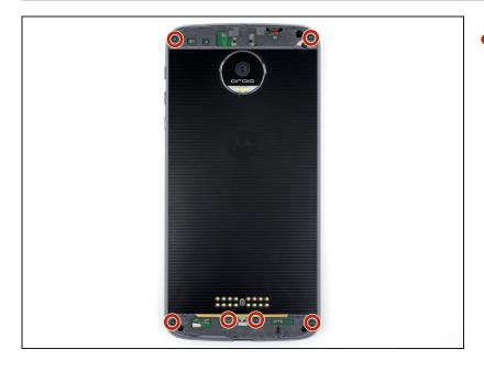
• Remove the six 4 mm T3 Torx screws securing the display assembly.
