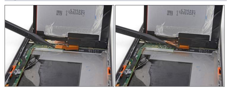
• Use the tip of a spudger to lift the battery connector up out of its socket on the motherboard.
