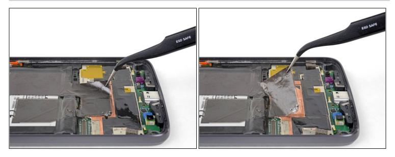
• Use <u>tweezers</u> to peel the black tape on the top of the battery up from the motherboard EMI shielding.
