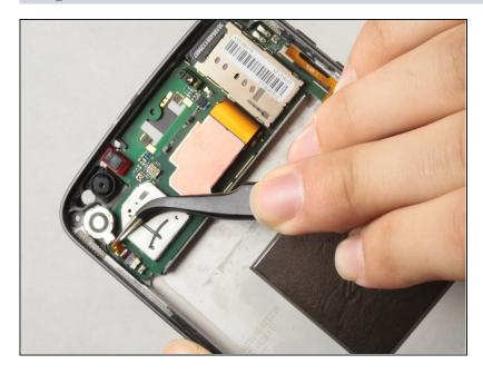
• Use <u>tweezers</u> to flip open the ZIF connector and remove the vibrator ribbon cable.
