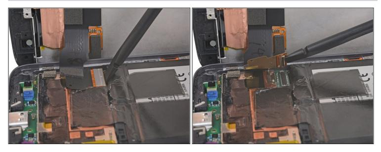
• Use the flat end of a spudger to lift the display cable connector up out of its socket.
