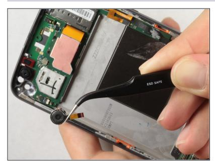
• Pry the vibrator motor from its position.
