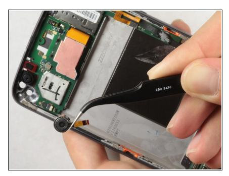
Pry the vibrator motor from its position.
