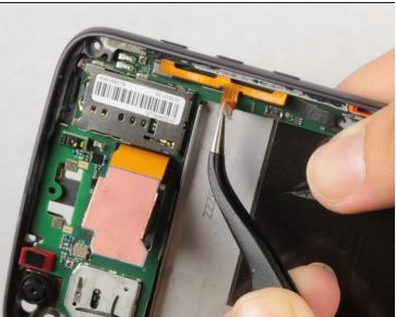
• Remove the golden connector attached to the volume buttons with a pair of tweezers.
