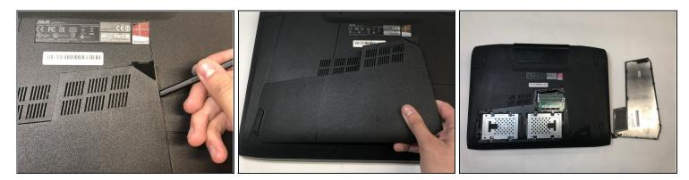
• Use the nylon spudger to remove the back center panel.
