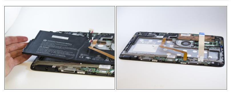
Carefully remove the battery without pulling the copper information transmitter out.
