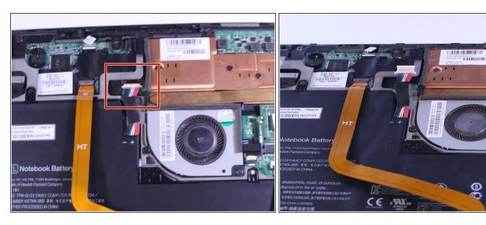
Unplug the bound (red, white and black) wires connecting the battery and the motherboard.
