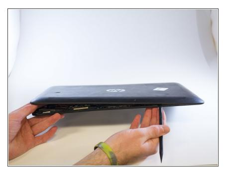
Gently use the black nylon spudger to pry the back casing from the screen until it snaps apart.
