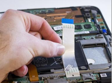
• Flip the gray latch back and remove the blue and white band of wires from the green motherboard.
