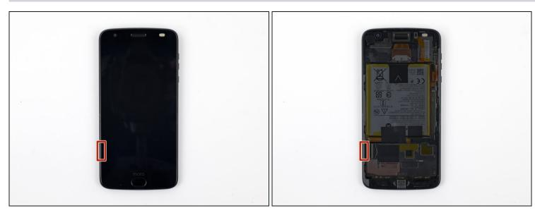
When separating the left side of the screen assembly, take care to not snag the display cable located on the left edge near the bottom of the display.
