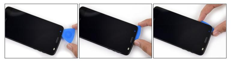
Insert an opening pick as deep as possible under the top left corner of the screen assembly to slice through the left patch of adhesive.
