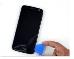
• Slide your opening pick all along the right side of the device to release the clips and adhesive securing the screen assembly.
