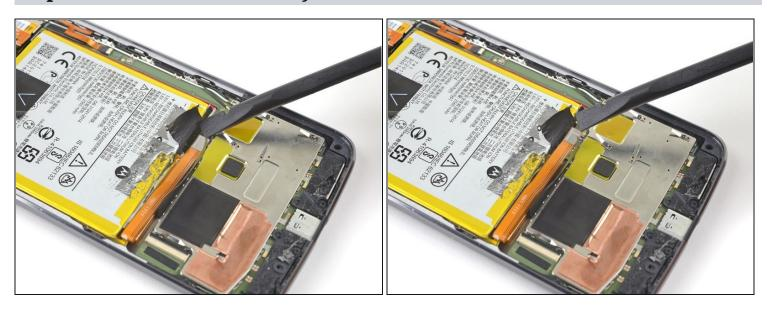
• Use a spudger to pry up and disconnect the battery connector.
