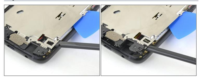
• Insert the flat end of a spudger under the lower right edge of the midframe and pry up to release the midframe clip.
