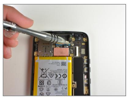
• Remove the T3 screw that is holding in the motherboard.
