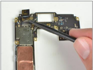
• Now use the flat edge of a spudger to carefully disconnect the camera from the motherboard.
