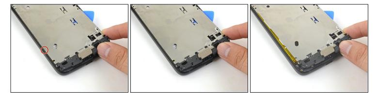
• Grasp the lower edge of the midframe and pull the edge slightly to the right, to clear the metal midframe clip.
