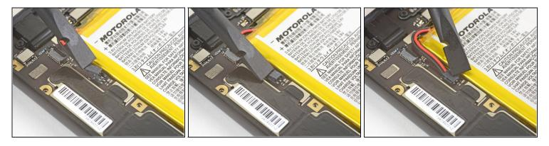
To re-connect the battery, align the connector on top of the socket, and press it down with your finger or a spudger.
