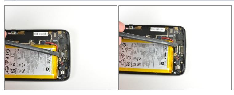
Use flat side of spudger to pry up connector near the bottom of the device.
