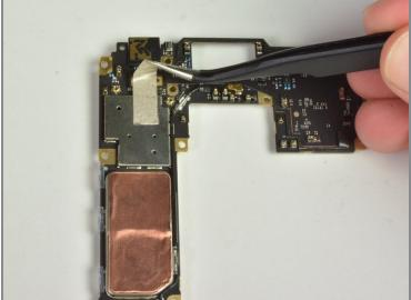
Now carefully peel off the tape on the back of the camera with tweezers.
