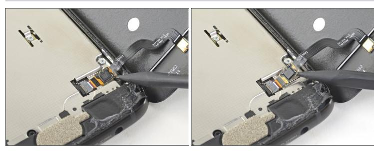
• Slide the point of a spudger underneath the fingerprint sensor cable and gently pry up to loosen the cable from the phone.
