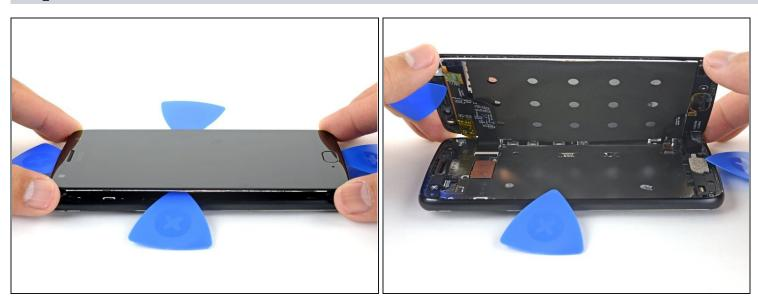
⚠ Do not try to remove the screen yet—it is still attached to the phone by delicate flex cables.
