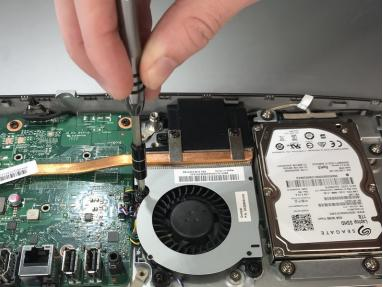
Remove the three screws that secure the fan.
