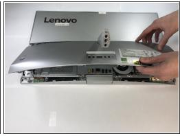
• Locate the slot on the right side of the computer next to the screw hole. Use a plastic opening tool or spudger to pry off the rear cover. (Don't be afraid to use a little force.)
