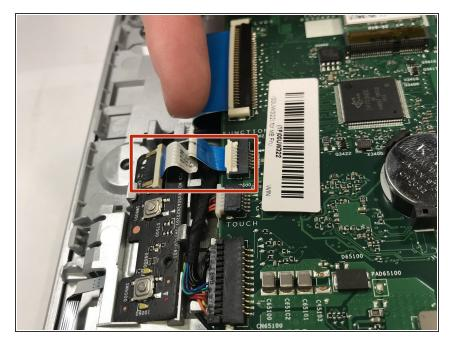
Locate the power switch board and the tan colored tab on it holding the blue and white ribbon cable down.
