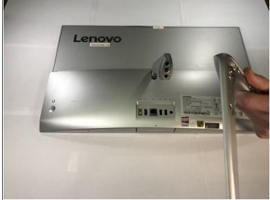
• Remove the monitor stand screw in the bottom of the stand, and remove the stand completely.
