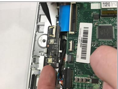
Slide the power switch cable out of its slot in the direction shown, making sure to lift up the end carefully.
