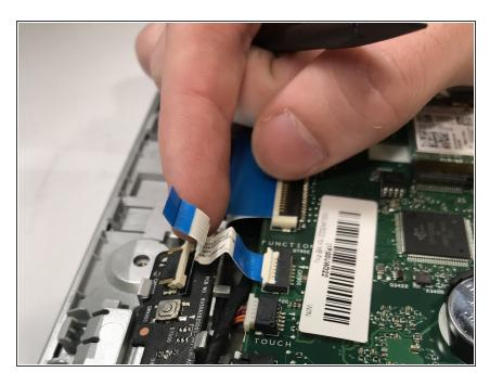
Pull the tab towards the blue and white ribbon cable to open it. Pull the cable out of the power switch board.
