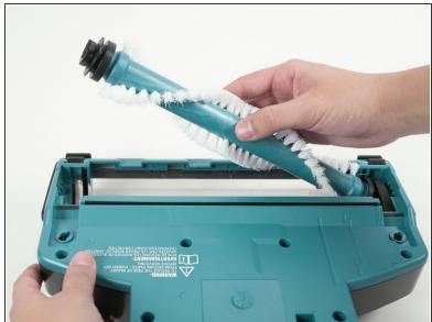
Grasp the brush roll firmly and pull up to remove the brush roll.
