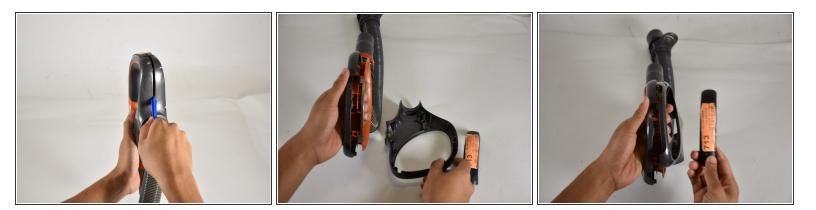
• Use a plastic opening tool to pry open the handle.
