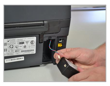
Grab the base of the colored, braided cable and pull it out of the AC Power Adapter.
