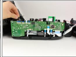
• Detach all the cables by gently pulling on them at their base in the direction of origin (for top connectors pull up and for bottom connectors pull down).
