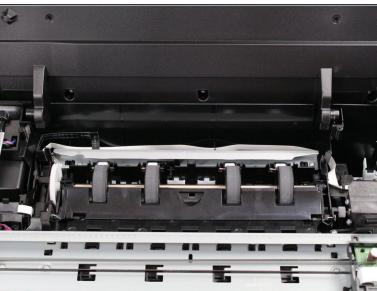
Grasp the gray lever of the black plastic cover of the rollers and gently pull the lever up and to the right.
