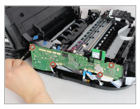
Remove the four 7 mm screws from the motherboard by placing the Torx 9 screwdriver in the screw slots and turning counterclockwise.
