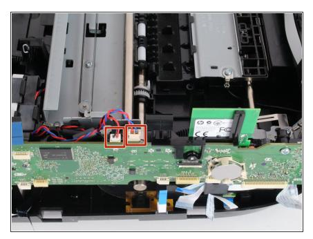
Remove the last two connectors found at the top of the motherboard by grasping the tan portion adjacent to the motherboard and pulling up.
