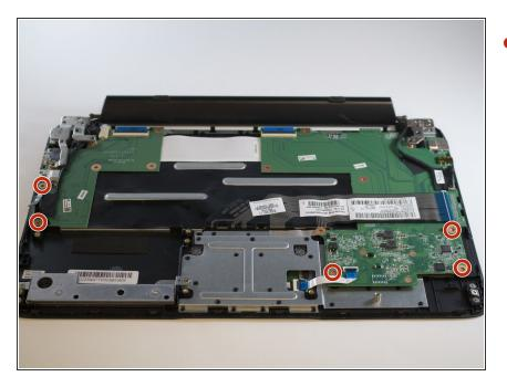
Remove five 5.0 mm Philips #00 screws from the green circuit boards.
