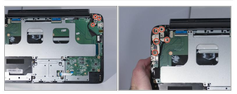
• Remove the eight 6.0 mm Philips #00 screws from the two silver holds.
