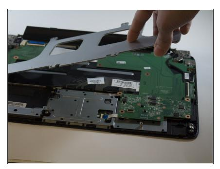
• Lift the metal brace and remove it from the device.
