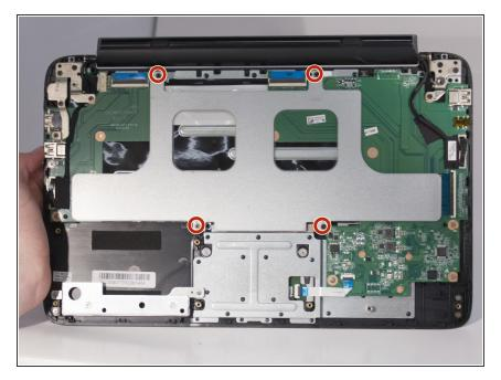
• On the silver metal brace, remove the four 6.0 mm Phillips #00 screws.
