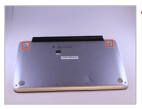
Remove the two rubber feet closest to the black hinge.
