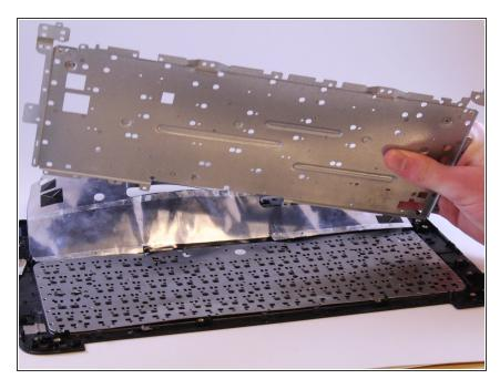
• Remove the metal plate to reveal the keyboard.
