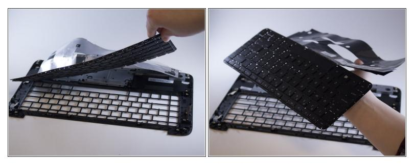
• Remove the keyboard from the device.
