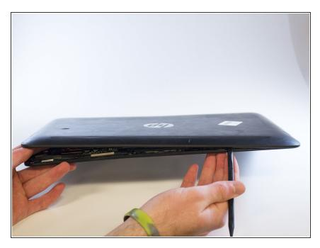
Use the black nylon spudger to carefully remove the back of the laptop from the screen.
