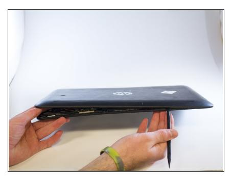
Remove the back of the laptop screen using a black nylon spudger.
