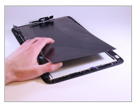
After you get some space at the top of the screen, proceed by using a thin board to gently remove the screen from the frame.
