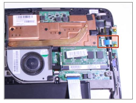
Remove the band that is attached to the circuit board, located on the right side.
