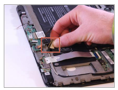
Detach the wires located just above the bigger green circuit board.
