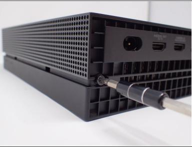
Use a T9 Torx screwdriver to remove the 13mm screw which is under and to the left of the power input.
