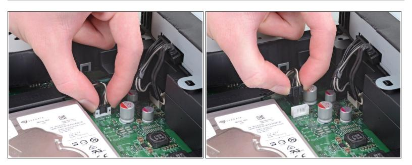
Unplug the bundled cable connector connecting the hard drive to the motherboard by pulling directly upward.
