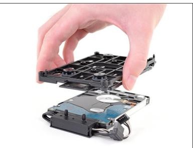
Lift the mounting bracket off the hard drive.
