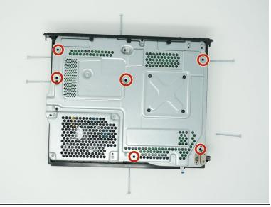
• Use a Torx T9 screwdriver to remove the six 47mm long screws, which attach the bottom side of the outer case.
