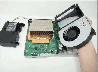
Remove the cooling system by lifting it vertically off of the motherboard.
