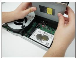
Lift and rotate the BD drive to reveal the wires that connect it to the motherboard.
