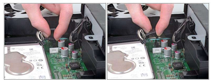
Unplug the SATA cable connecting the hard drive to the motherboard by pulling directly upward.
