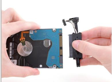
• Unplug the hard drive connector from the hard drive by pulling parallel to the length of the drive.
