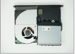
Remove the metal casing by pulling it upward, revealing the interior components of the device.
