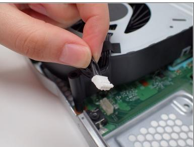
Disconnect the plastic wire connector from the motherboard.
