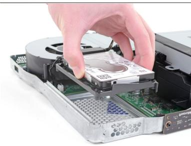
Lift the hard drive assembly up out of the upper metal case.
