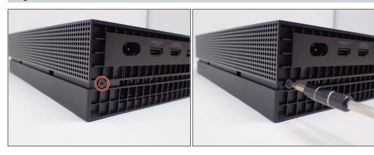
Use a T9 Torx screwdriver to remove the 13mm screw which is under and to the left of the power input.
