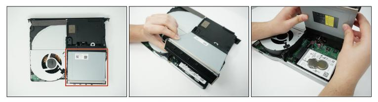
• Lift and rotate the BD drive to reveal the wires that connect it to the motherboard.
