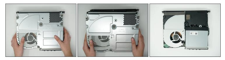
Remove the metal casing by pulling it upward, revealing the interior components of the device.
