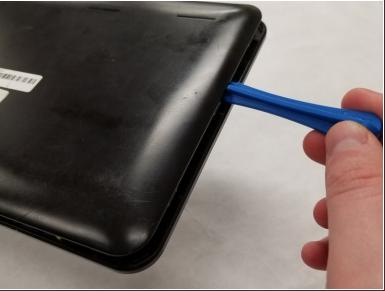
• Gently apply pressure to the back of the device where the backing case and screen meet.
