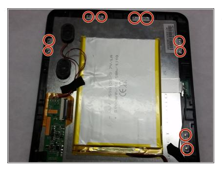
Remove ten 25mm JIS #00 screws securing the screen.
