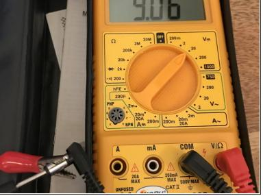
• Put back the screw, the sticker and with a multimeter check that you've got the desired voltage output, in the correct polarity! To reassemble your device, follow these instructions in reverse order.
