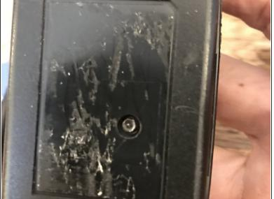
Remove the sticker to be able to access the screw that holds the two halves of the casing together
