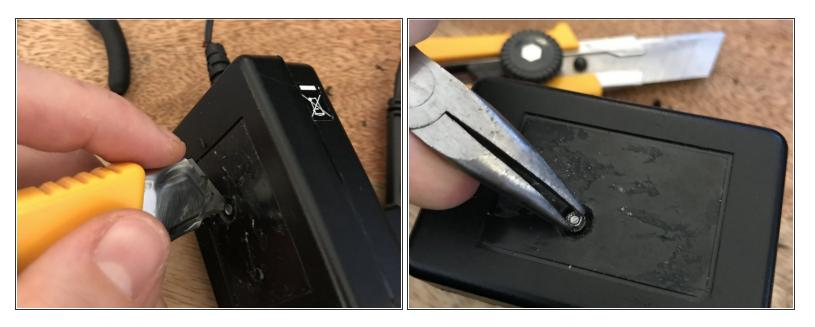
The screw is tiny and requires some kind of tiny wrench that I don't have, so I made the whole a bit bigger around it to be able to unfasten it with regular pliers.
