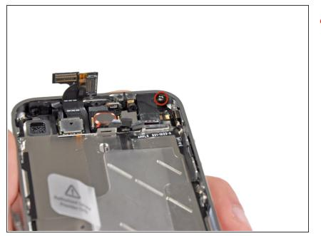
Remove the 1.5 mm Phillips screw securing the front panel near the headphone jack.
