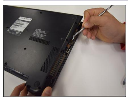
Next, move around the edges of the computer with the metal spudger prying off the casing. You should hear clicks as you do this; this is not the casing breaking, it is just popping off.
