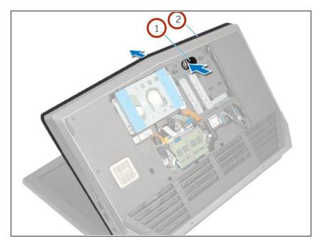
Lift the computer base slightly and push the palm-rest assembly through the slot on the computer base to release the tabs on the palm-rest assembly.
