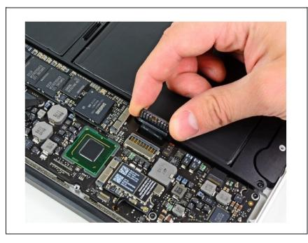
Reconnect the battery. Wait for few seconds and reconnect the battery.
