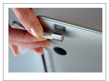
Plug the charger. You should see the cooling fan working, even though the led of the MacBook is closed (a sign that the MacBook is switching on).
