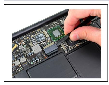
Disconnect the battery. Use your figures or a plastic tool to disconnect the battery connector.
