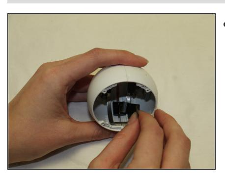
Reach inside the circle and pull the ribbon cable free from the device.
