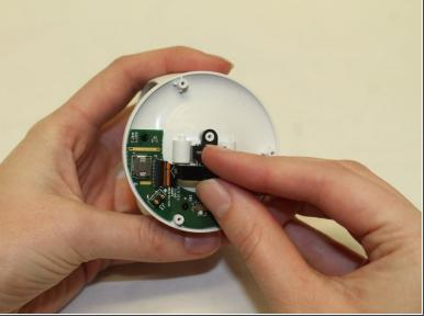
Gently pull the ribbon cable loose from its connection to the base.
