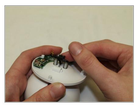
Remove the black plastic connector and the two springs from the base of the device.
