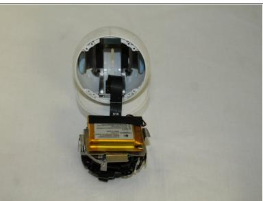
Gently remove the lens/battery bundle from the base of the circle, being mindful of the ribbon cable.
