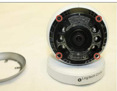
Remove the four 3mm Phillips #0 screws that hold down the second ring.
