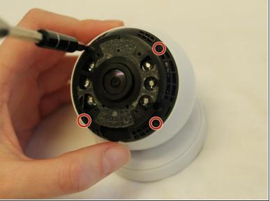
• Remove the four 3mm Phillips #0 screws that hold down the first ring.
