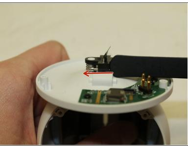
Slide the push pin holding the plastic connector/ribbon cable in place out on both sides.
