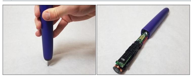
• Put the metal head on a solid surface with handle perpendicular to the surface. Firmly, yet gently, push down until the internals start to slide out.
