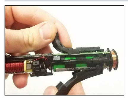
Remove rubber covers from the top of the motherboard and the back of the battery.
