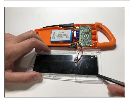
Using the spudger, pry the solar panel off the cover.
