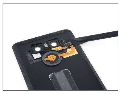
Use the blade of a halberd spudger to pry the rear button chip off of the rear case.
