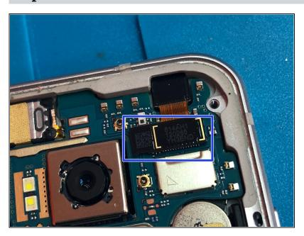
• Use the flat end of a spudger to disconnect the front camera.
