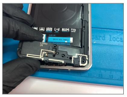
• Remove loudspeaker assembly.
