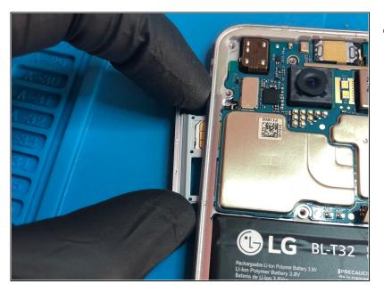
Insert a SIM card opening tool into the small hole on the left side of the phone and remove the SIM card tray.
