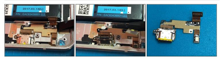
• Use the flat end of a spudger to remove the adhesive securing the USB-C charge port to the frame.
