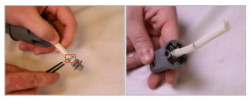
Use your tweezers to remove the metal ring holding the hose to the plastic end piece and replace the hose / bit as needed.
