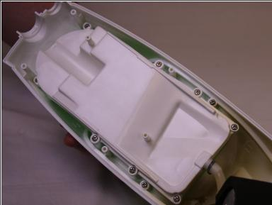
Start by gently moving the midframe from the top portion of the panel to expose the bottom portion of the mop's water tank / bladder.
