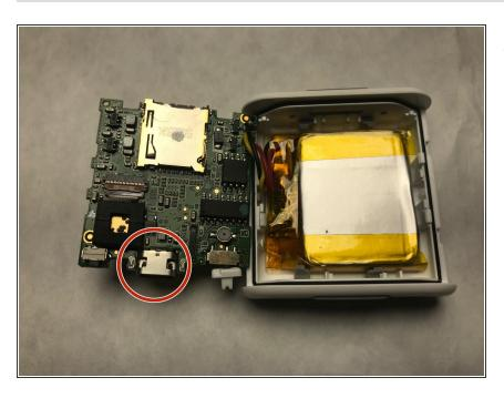
• With the Micro USB port exposed, part can be replaced with advanced soldering and circuitry.
