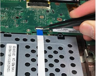
• Unlatch the data cable by using tweezers to lift the white tab and release the cable.
