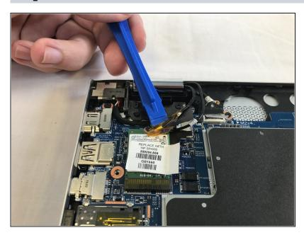
Use the plastic opening tool to disconnect Disconnect the two cables attached to the wifi
