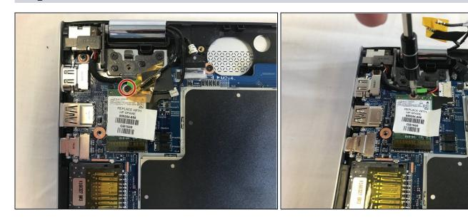
• Use a PH0 tool bit to remove the one 2.8mm screw.
