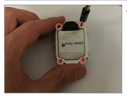
• Use the T5 head on the iFixit screwdriver to unscrew the four screws on the back of the watch's face.
